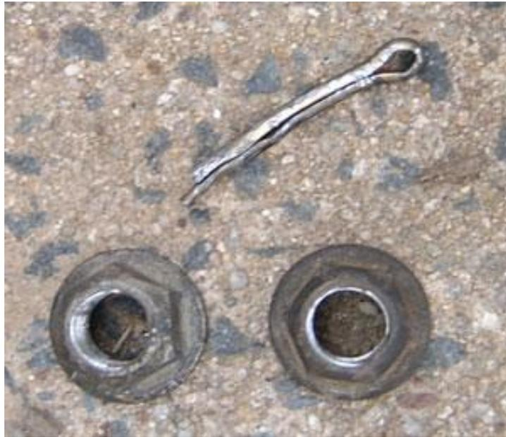
Step 8. Loosen the crown bolt. If you have a rattle gun, this bit is fairly easy. If not, get someone to put their foot on the brake while you attack the nut with a socket. Once you have loosened it, wind it off most of the way (as pictured below).
