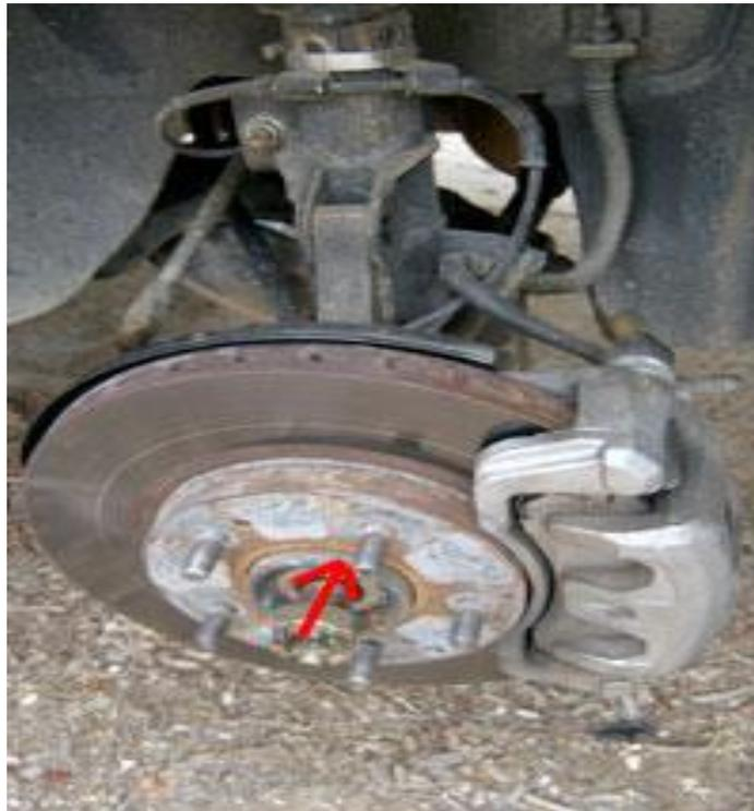
Step 9. Give the nut a tap with a hammer. The shaft should move in the direction of the arrow.
