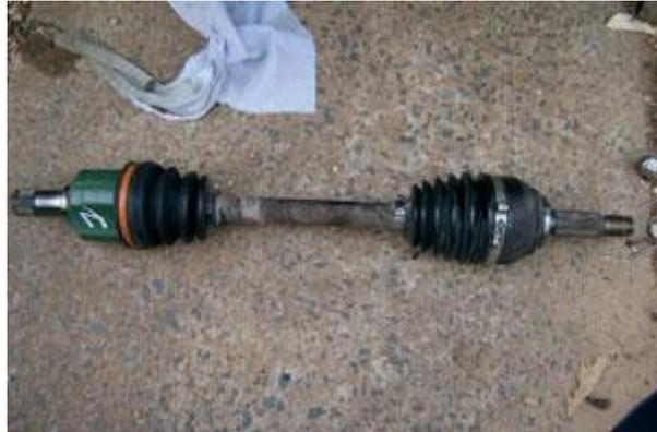
Before we start, it is worth mentioning that the drive shafts on an FTO with ABS are different to those on an FTO without ABS. If you happen to require new drive shafts, make sure you procure the correct ones.
