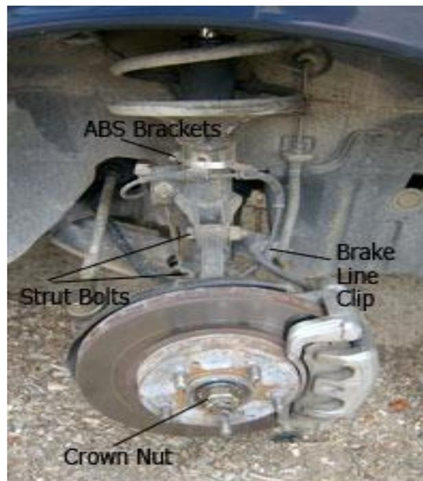
Step 4. Remove the ABS brackets or detach the ABS line from the brackets. Mine are held on by a hose clamp, but this is not always the case. NOTE: If you dont have ABS on your FTO, ignore this step.
